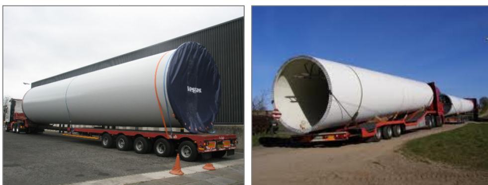
Figure 1.7. Transportation of wind turbine's tower
