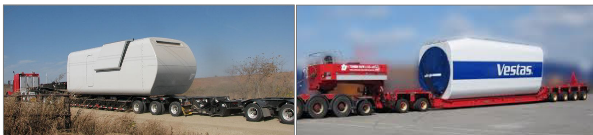
Figure 1.6. Transportation of wind turbine's nacelle
