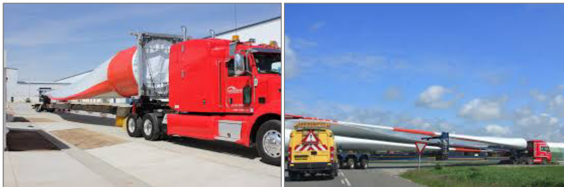
Figure 1.5. Transportation and discharging of the wind turbine blades
