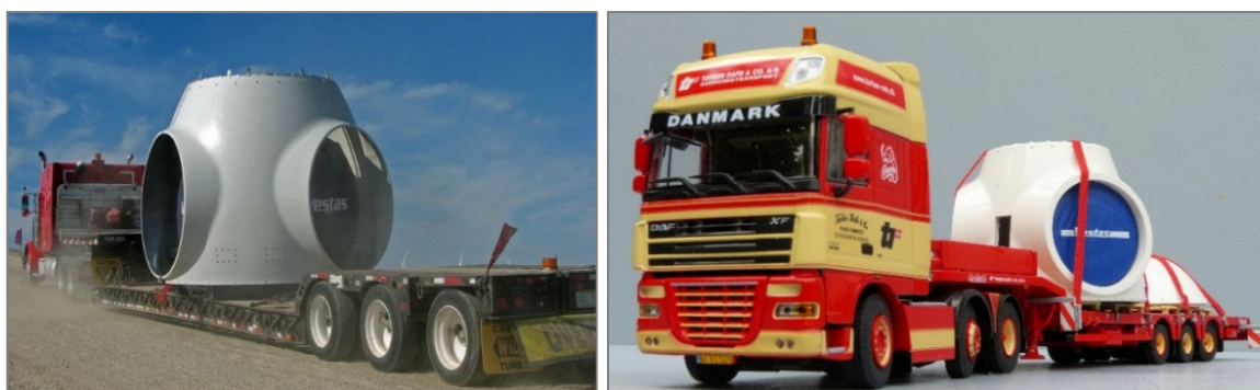
Figure 1.8. Transportation of wind turbine's hub
